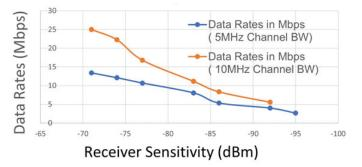
Figure 9. Receiver sensitivity and data rates.
