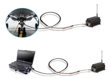
Figure 2. Overall setup of the aircraft to ground wireless transfer.
