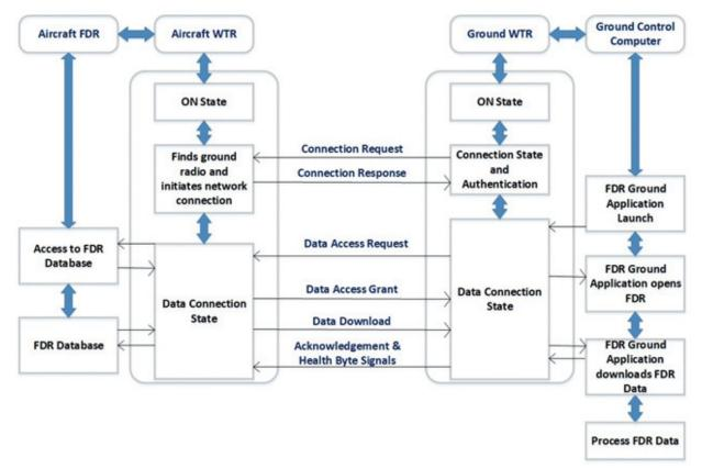
Figure 6. Data transfer state machine.
