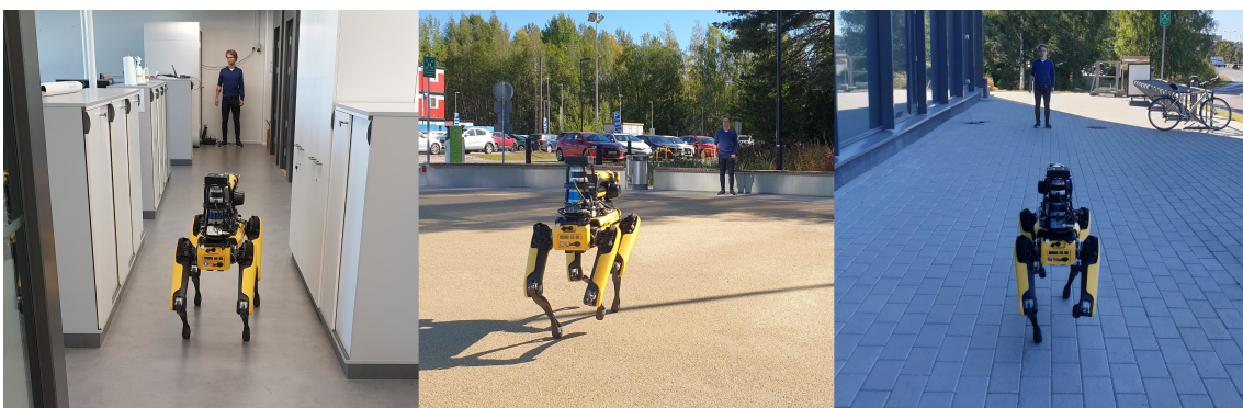
Figure 8: Distance related measurements with Spot at different locations. Left: Indoors location at an office. Middle: Outdoors location in direct sunshine. Right: Outdoors location in the shade.
