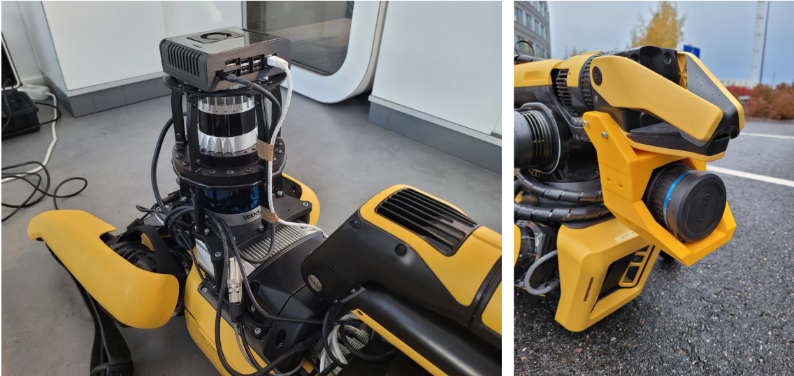
Figure 4: The devices attached to Spot. Left: From top to bottom: NVIDIA Jetson Xavier NX Development Kit in a 3D-printed casing, Ouster OS0-128 LiDAR, Velodyne Puck LiDAR, and Spot CORE. The network switch is in the bottom right of the image below the Spot Arm. While the Velodyne Puck was used by Spot for sensing the environment and the Ouster OS0-128 could be used for performing additional scans of the environment, the two LiDARs are not directly related to this work. Right: Flir thermal camera attached to the arm.
