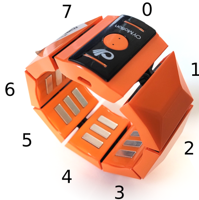
Figure 3: The gForcePro+ sEMG armband used in this thesis. The numbers indicate how the eight sets of dry electrodes are mapped to the eight channels of the device.
