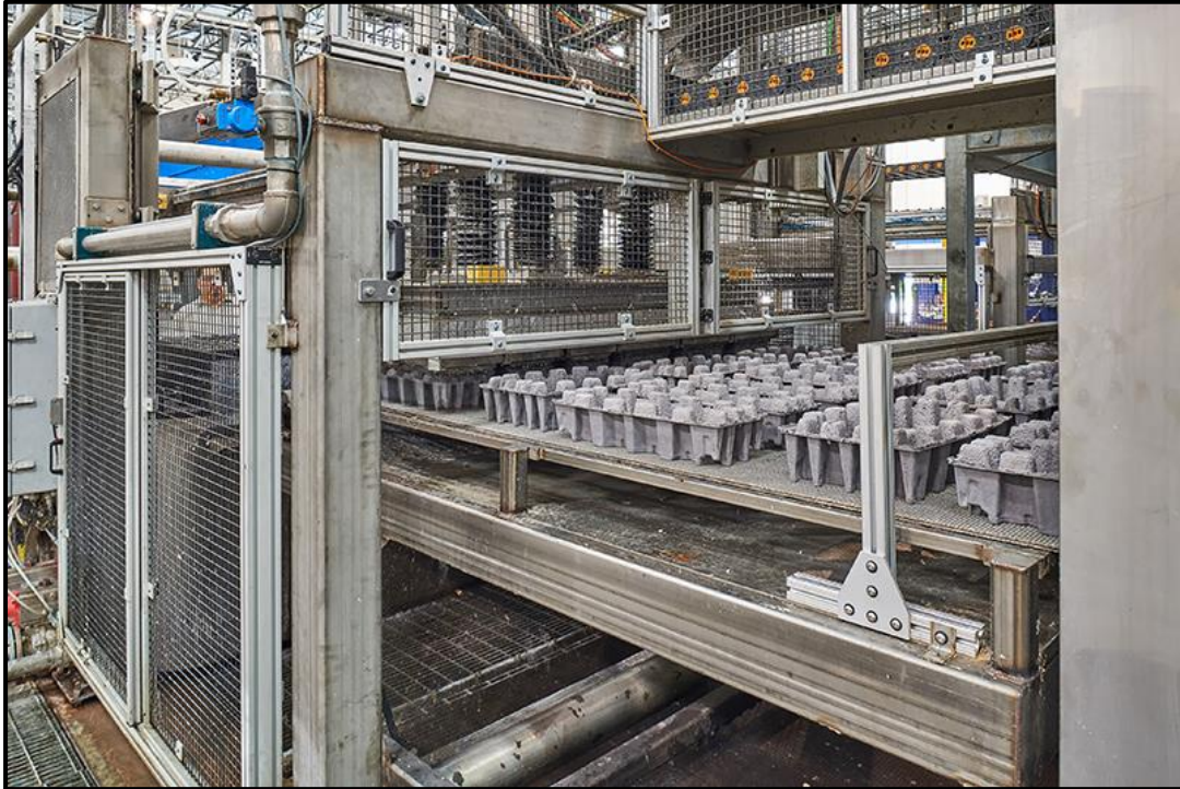
Figure 6: Part of the fiber-casting machine that produces egg trays (UFP Technologies, 2021)
