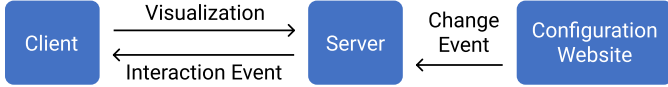
Fig. 5. This figure shows the framework of the prototype and relationship between client, server, and configuration website.
