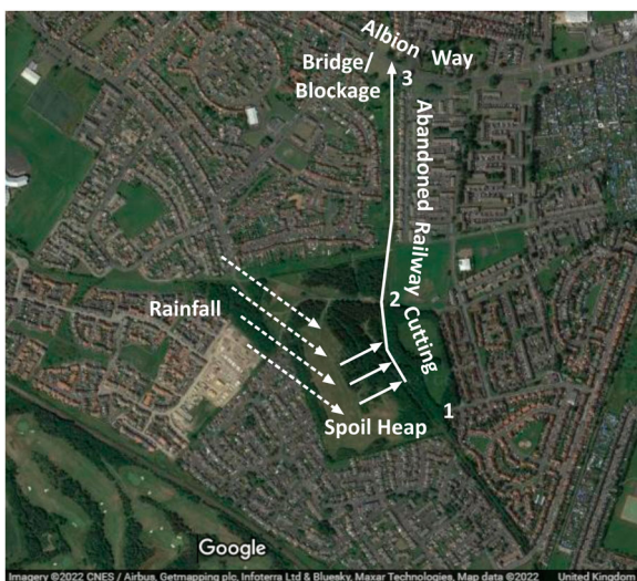
Figure 3. Water flows and flood extent as described by Northumberland County Council (2020). Images are available in colour online.
