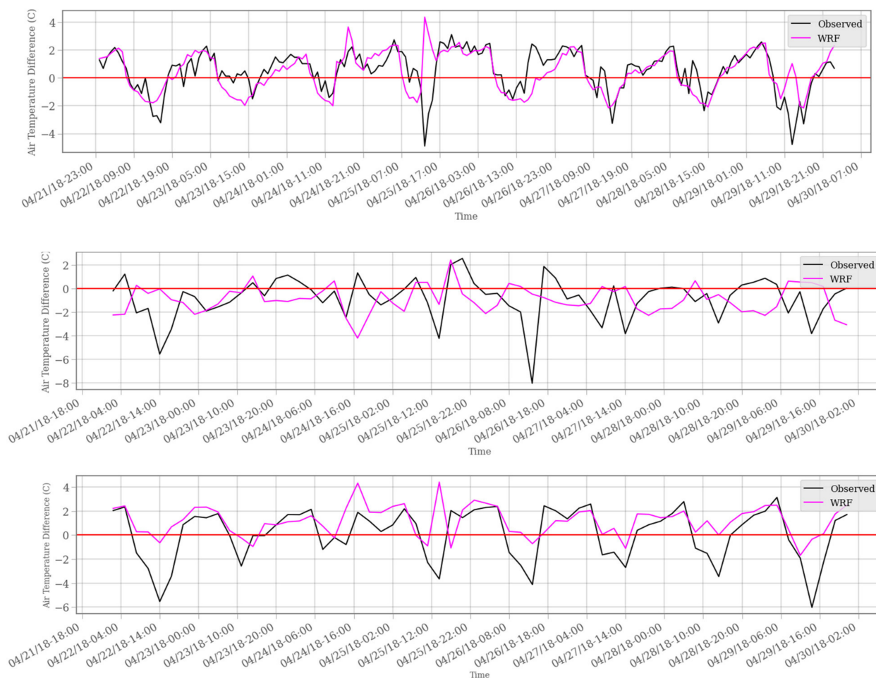
Figure 4. Temporal evolution of urban heat island intensity of observed and WRF simulation for NAIA ( top ), SGQ ( center ), and Manila Port ( bottom ). Positive values indicate higher urban temperature while negative values indicate higher rural temperature.
