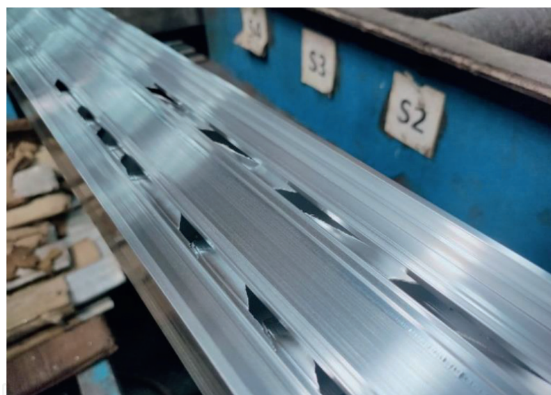
Figure 4. Bubble or blister appearing on extrudate surface.
