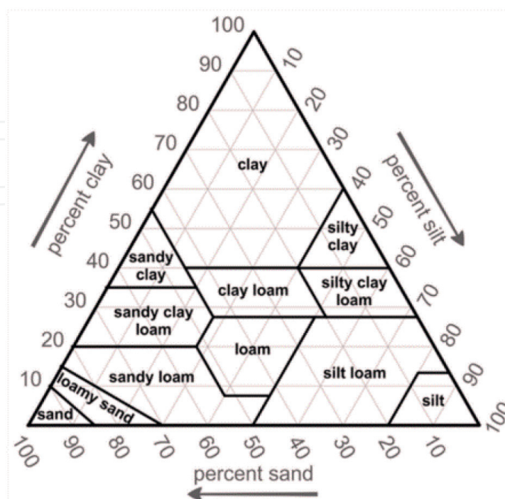
Figure 1. Soil's texture triangle classification diagram [14].
