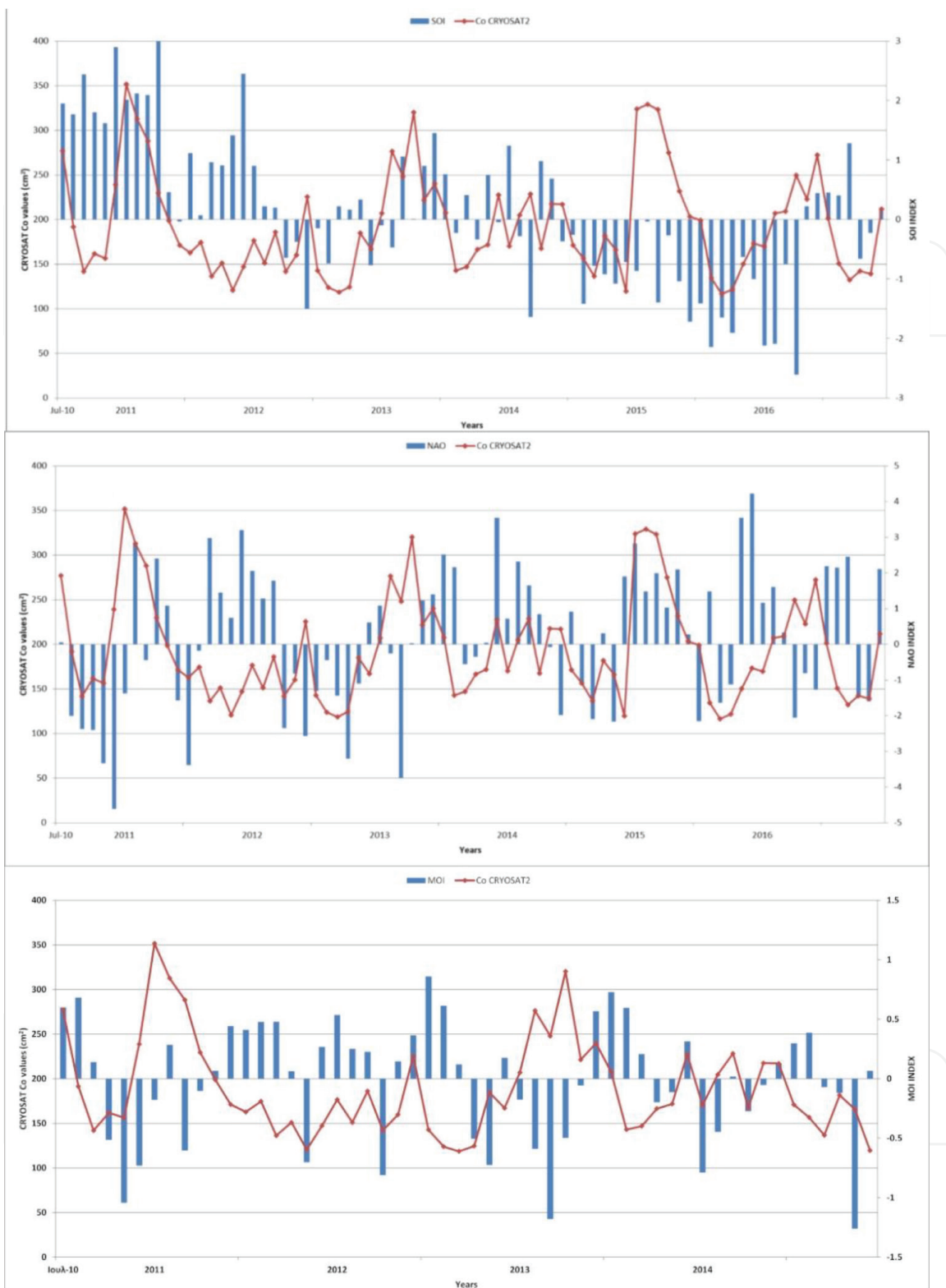
Figure 9. Cryosat-2 SLA variances fluctuations from 2008 to 2017 and correlation with SOI (up), NAO (middle) and MOI (bottom).
