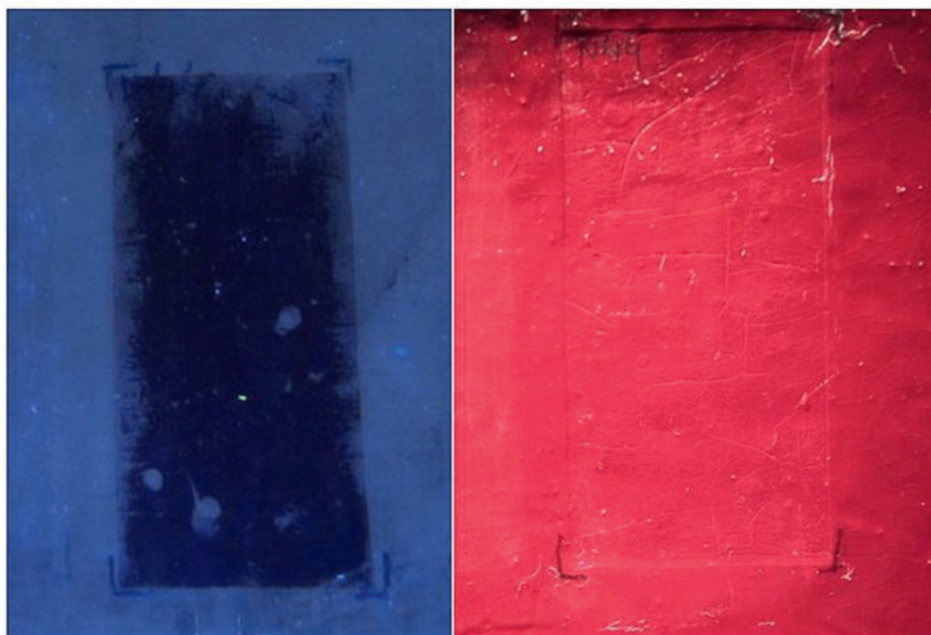
Figure 6. Photographs with UV/(left) and oblique visible light (right) of the standard sample varnished with mastic on cadmium red oil after cleaning with formulation N44.
