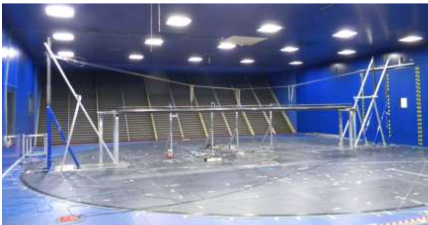
Figure 4 The complete model in the wind tunnel test section
