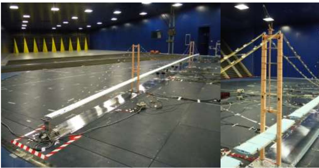
Figure 3. The full bridge aeroelastic model in the boundary layer wind tunnel (left) and a detail of one construction stage analyzed (right)
