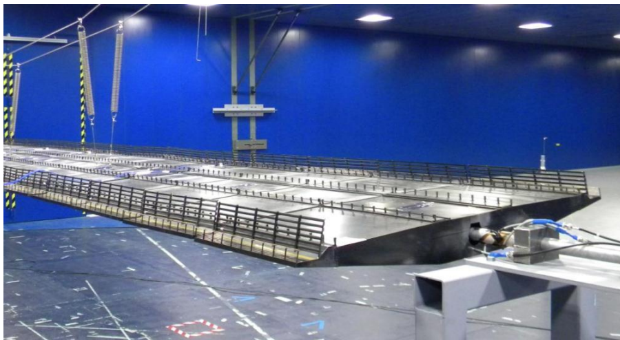
Figure 12. Aeroelastic multi-modal deck model of the BB3 in the POLIMI wind tunnel scale 1:50
