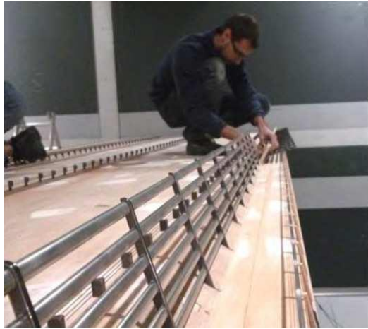
Figure 14. Rigid deck model of the BB3 in the CSTB wind tunnel scale 1:25
