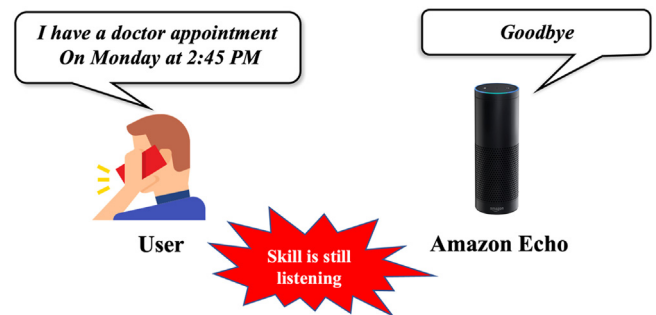
Fig. 3. A skill faking termination: User shares personal information thinking skill is terminated [16].
