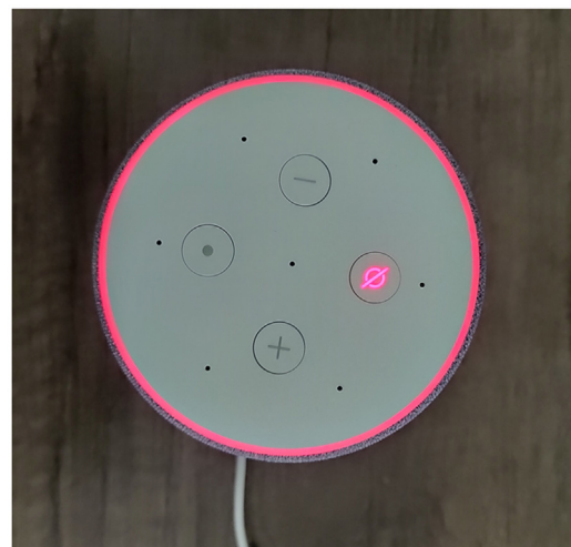
Fig. 8. User turn device mic off while revealing confidential information. Echo's LED light turns red while mic is off.
