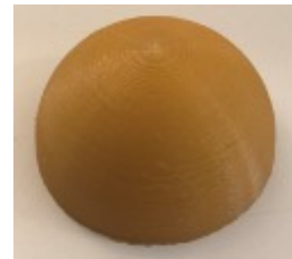
Fig. 6. Photo of the physical half ball-shaped object printed by LulzBot TAZ FDM printer.
