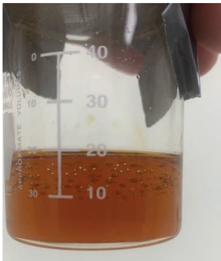
FIGURE 1: LIQUID PI PREPARED FROM 22 WT.% OF POLYMER RESIN DISSOLVED IN NMP.
