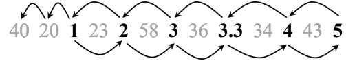
Fig. 3. TSC17 looks for bi-directional connections between subsequences. A left pointing arrow links a subsequence to its left nearest neighbor (LNN), while a right pointing arrow links a subsequence to its right nearest neighbor (RNN). Here the chain breaks at 1, as LNN(1) = 20 but RNN(20) = 23 \neq 1 .
