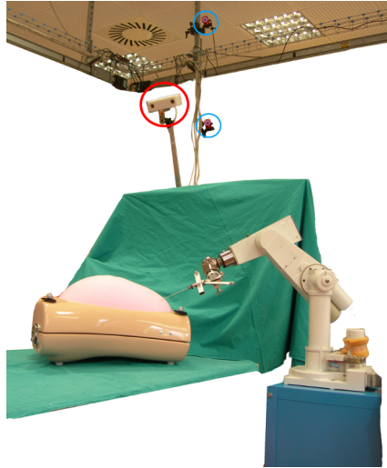
Fig. 1. In this picture is possible to see the devices that compose the test case. There is one robot that move the surgical needle and two trackers that save the trajectories
