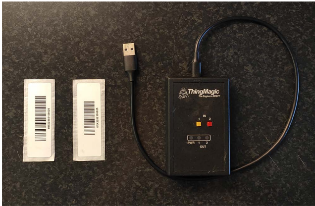
FIGURE 3. ThingMagic M5EC RFID reader and non-modified commercial UHF RFID tags.
