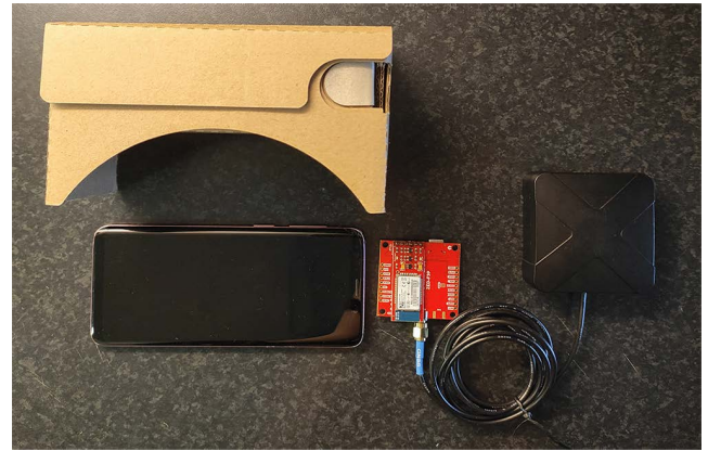
FIGURE 4. Cardboard VR Goggles, Android Smartphone, SparkFun GPS-RTK2 rover with bluetooth module and patch antenna.
