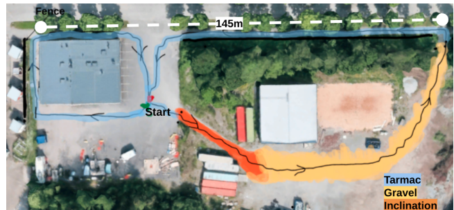
Fig. 6: Outdoor experiment 1: top of view of the trajectory to test the effect of various mounting positions and terrain types.
