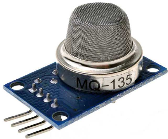
FIGURE 5 MQ135 air quality sensor used to determine the changes of rainbow trout's head and meat odor
