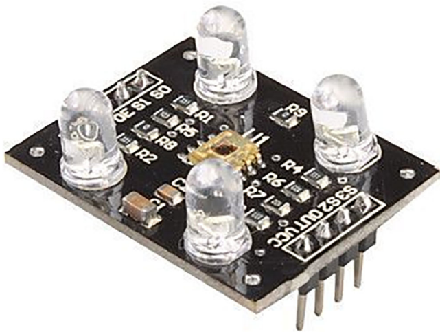
FIGURE 4 TCS3200 color sensor used to determine the rainbow trout's head and meat color
