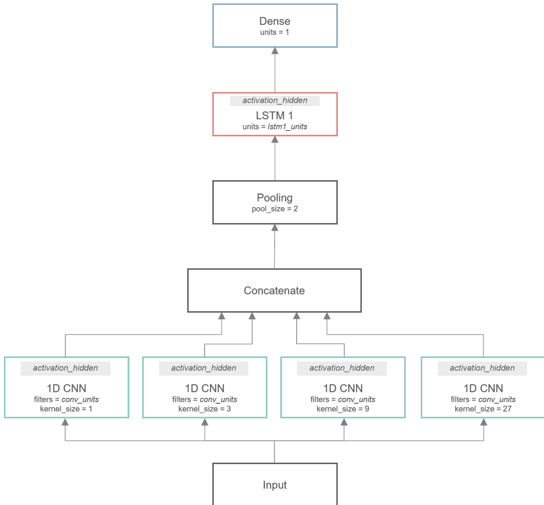
Figure 3.8: A sample 1DCNN-LSTM network architecture.
