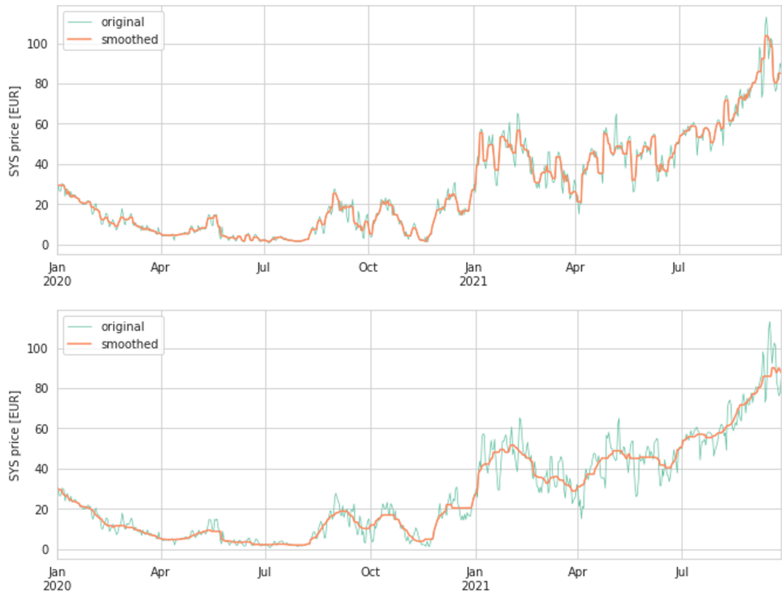
Figure 3.6: Input data transformation—various levels of smoothing applied on the SYS price time series. The smoothed curve in the upper plot corresponds to the smoothing window of 5 samples, in the lower plot—the window of 21 samples.
