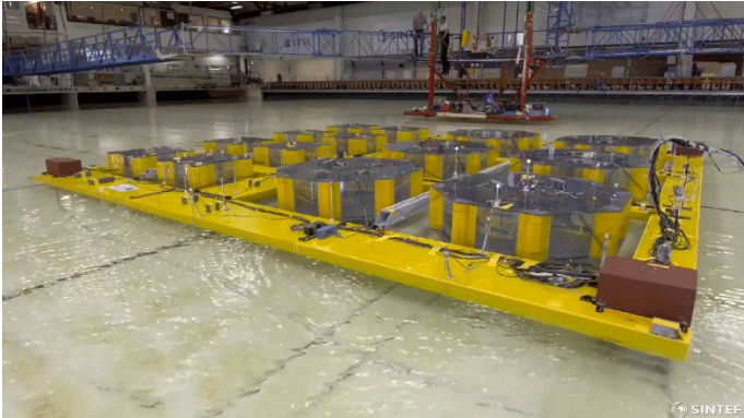
FIGURE 6: MODEL TESTING OF A FLOATING STORAGE FACILITY FOR USE IN SINGAPORE. CREDIT: SINTEF OCEAN
