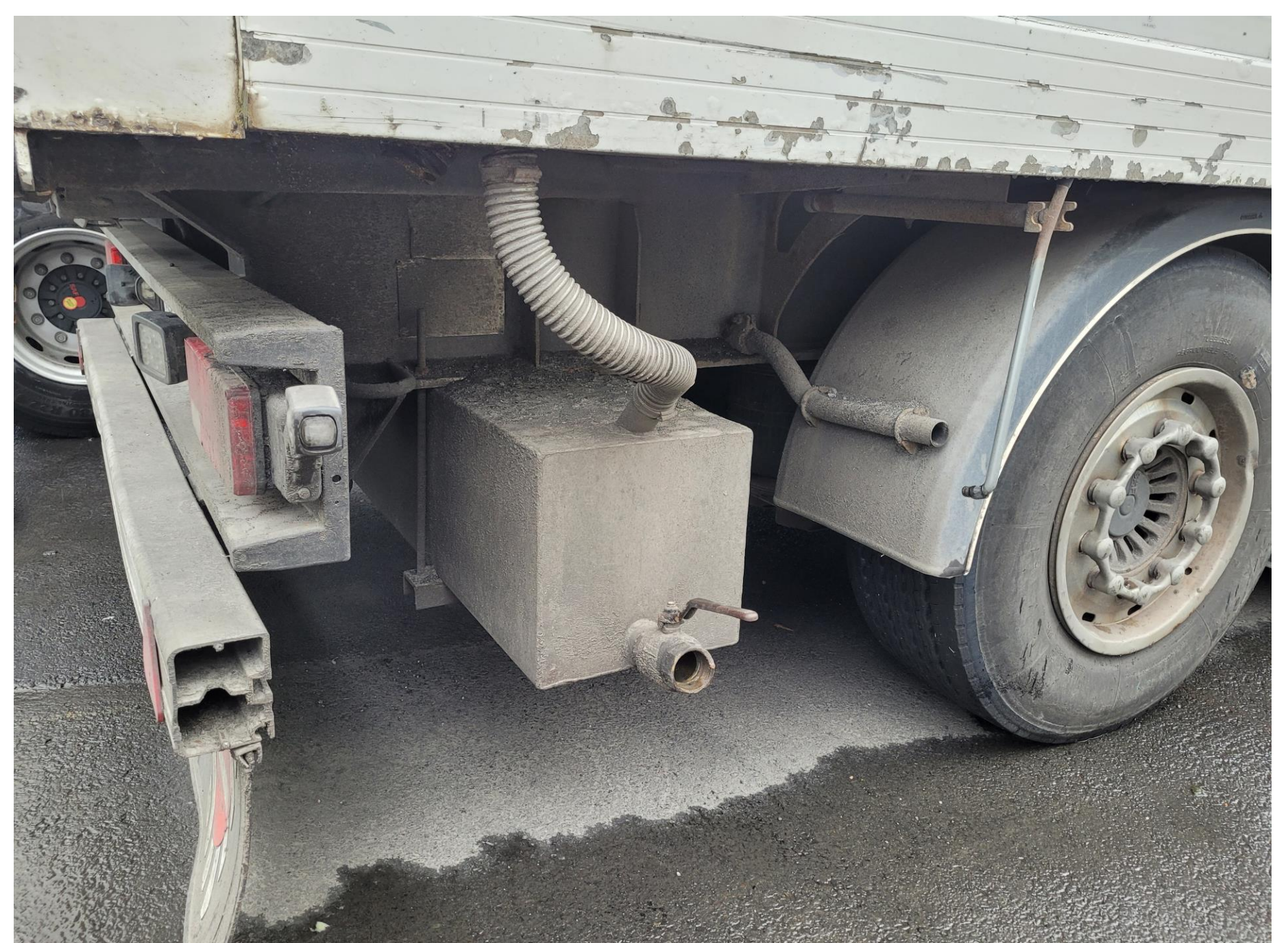
Figure 5. Example of meltwater collection system used in Iceland. Tanks differ in size and design.
