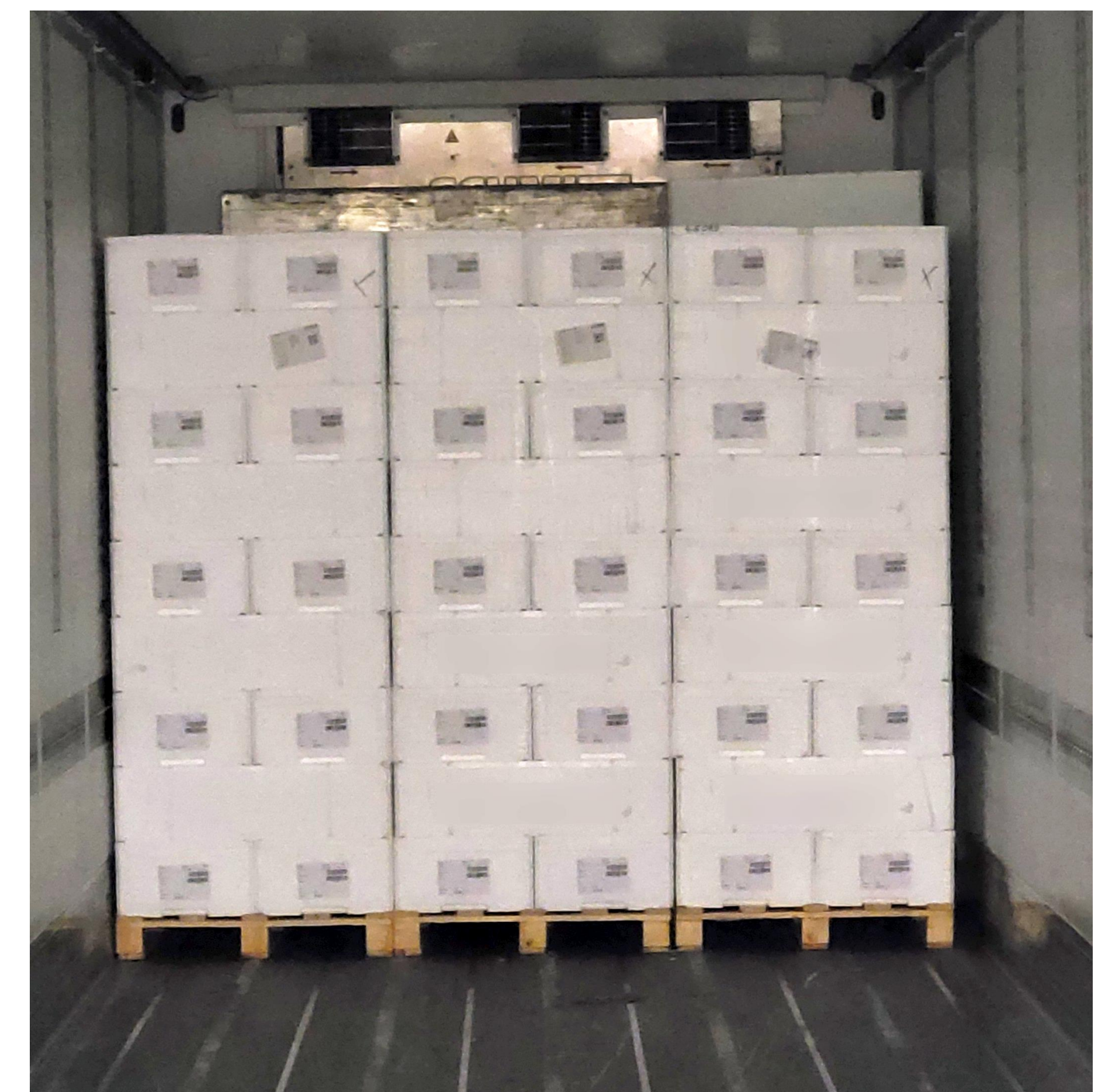
Figure 3. EPS boxes stored in semi-trailer, usually 33 pallets of 27 boxes each. Precise pallet alignment differs between loads.
