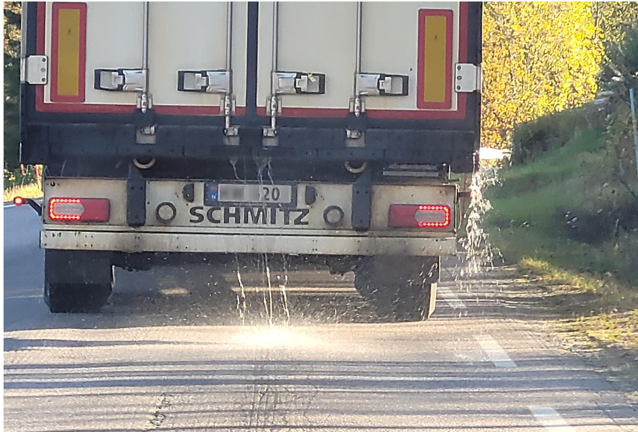
Figure 1. Example of meltwater draining during salmon transport 30 minutes after loading. The semi-trailer was pre-cooled and operating at 0 °C. Drainage shown here was limited to uphill sections and turns. The truck was caught in a routine inspection of the Norwegian Public Roads Administration shortly after where the inspector noticed no water draining.
