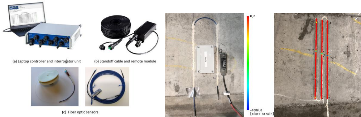
Figure 4 – a) Fibre Optic System. This platform is configured to measure standard “Rayleigh” High-Definition Fiber Optic Sensors (HD-FOS). HD-FOS operation is based on the measurement of the Rayleigh backscatter in optical fiber and delivers maximum spatial resolution for static and quasi-static applications. b) Installation of fibre optics in section where we also have a crack (LVDT) and a strain gage. c) Optical results from the FOS monitoring
