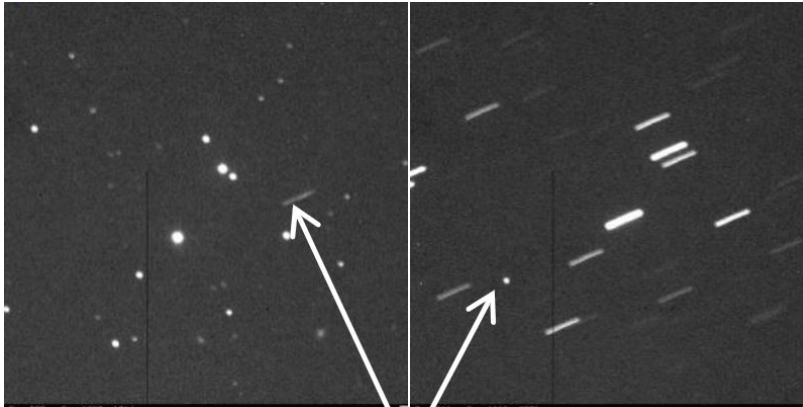
Figure 6: Comparison of sidereal tracking (left) to tracking at the rate of an object's motion (right) with the object's position noted, adapted from [16].
