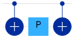
Figure 41: The physical gates used to encode \exp(-i\gamma C_{(u,v)}) . Here, the top qubit is qubit u and the bottom qubit is qubit v . The P gate has phase -\gamma .
