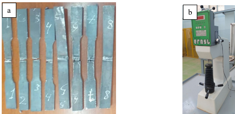
Fig 4 - (a) Samples used for tensile strength; (b) Ernst Rockwell hardness tester
