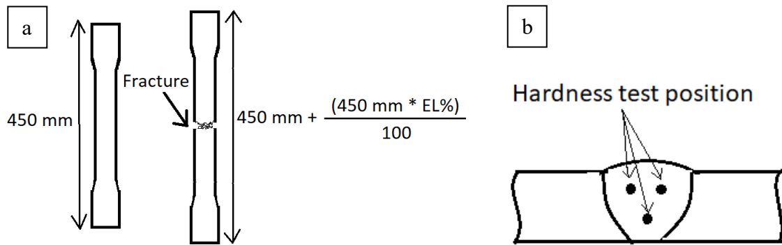
Fig 5 - (a) Elongation formula for tensile strength samples; (b) hardness-tested positions in welding
