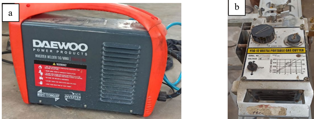
Fig. 2 - (a) Welding machine Daewoo Inverter Welder TIG/MMA; (b) Welding speed machine YSG-12
