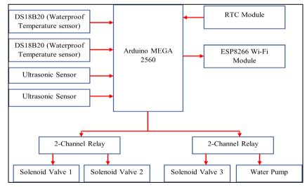
Fig. 2 - Block diagram design of the autonomous and monitoring system
