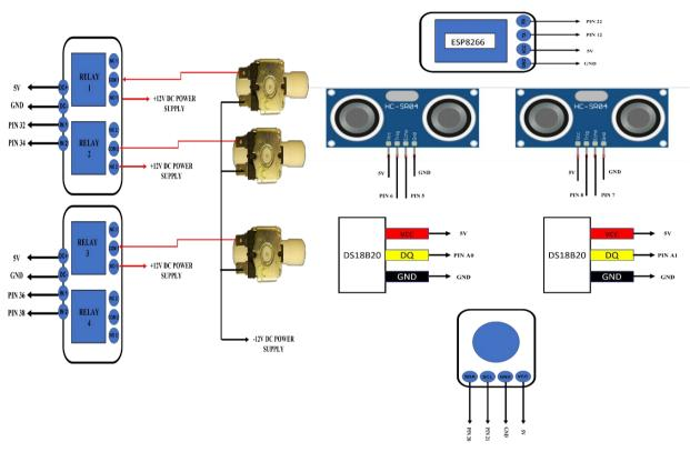
Fig. 5 - Components connection to Arduino Mega 2560 Pinout
