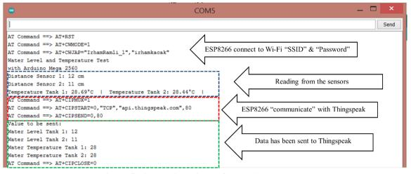
Fig. 7 - Serial monitor display for monitoring system
