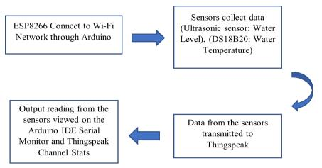
Fig. 3 - Monitoring Process communication to Thingspeak via ESP8266
