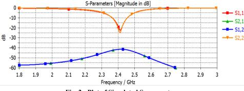
Fig. 2 - Plot of Simulated S parameters
