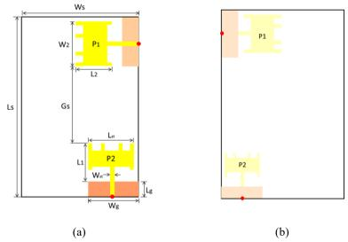
Fig. 1 - (a) The geometry of the designed antenna (front side); (b) The geometry of the designed antenna (bottom side)
