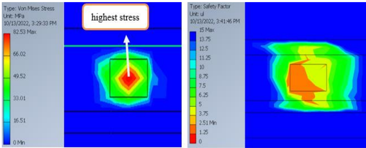
Fig. 4 - Left: Maximum von mises stress distribution; Right: Factor of Safety for rail surface
