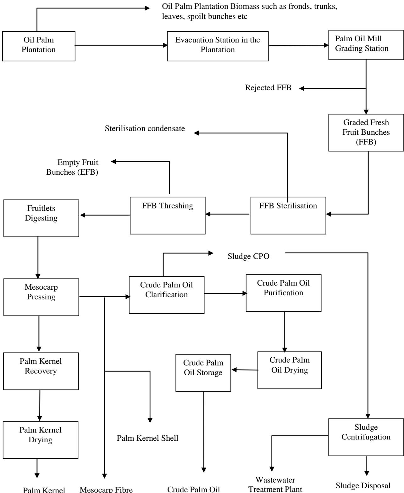
Fig. 1 – Palm Oil processing from the plantation to the mill
