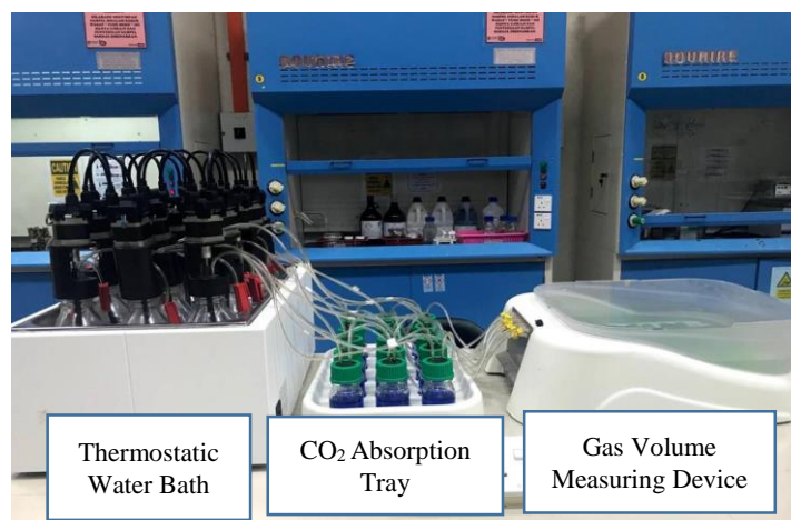
Fig. 3 - AMPTS II (only 5 reactors used for SMA testing)
