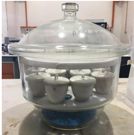
Fig. 4 - Desiccator containing crucibles to be cooled
