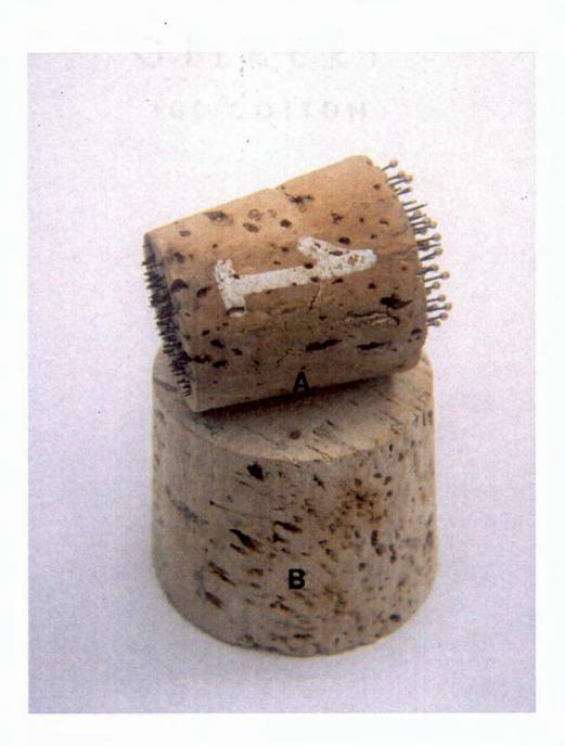
Fig. 1. Wounding tool: (A) Cork stopper with #1 insect pins used to wound adaxial leaf surface and (B) larger cork stopper used to support abaxial leaf surface while wounding.
