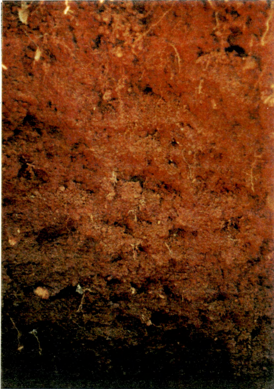
Plate 3. Picture of bridging voids, which averaged 1 cm in diameter, in spoil 1.
