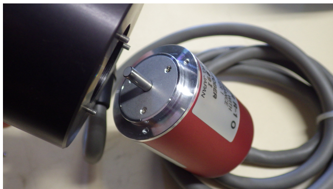
Figure 2.11: Laser rotary encoder that monitors the rotation speed of the scanner DC motor.
