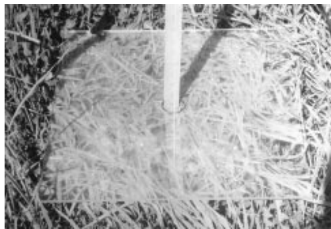
Fig. 2. The acrylic plastic plate meter being used to measure the bulk height of a grass-clover pasture.
