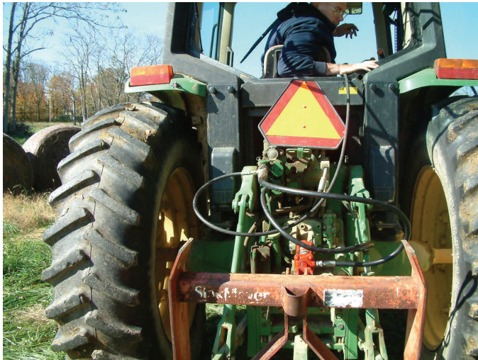
Figure 8 - Rear view of Cylinder as Top Link
