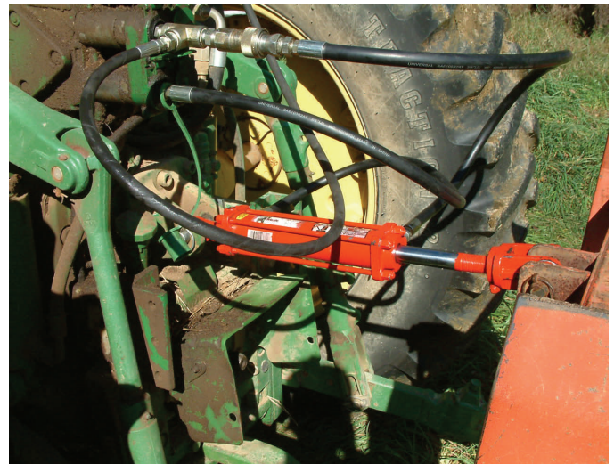
Figure 9 - Side View of Cylinder as Top Link
