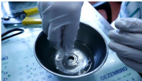
Fig. 5. Grease removal process from the bearings.
