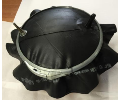
Figure 2: Equipment for impact tests with distributed load.
