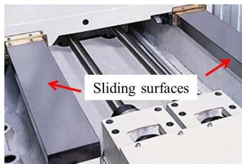
Figure 5.15 Photo of sliding surfaces of milling machine.
