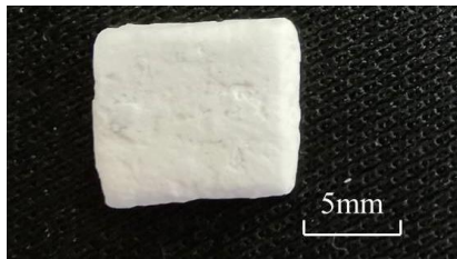
Figure 2.9 Diatomaceous earth chip before absorbing electrolyte.
