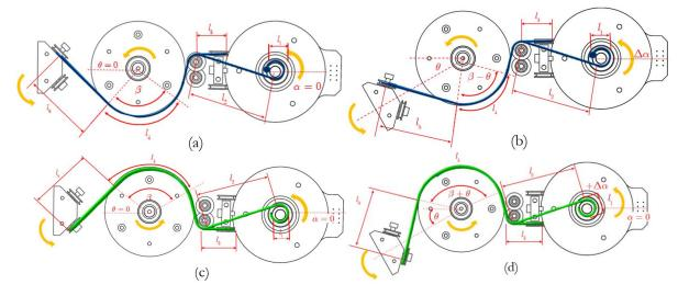
Fig. 4. Cables length of the mechanism at different stages when motor rotate in the counterclockwise direction. (a) blue cable at the initial stage. (b) blue cable at the arbitrary stage. (c) green cable at the initial stage. (d) green cable at the arbitrary stage.
