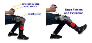
Fig. 9. Experimental setup for the active-assistive and resistive experiment.
