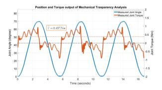
Fig. 11. The result of position tracking under no-load conditions for mechanical transparency analysis. The highest torque value is 1.02 Nm, and the RMS torque is 0.457 Nm. The positive torque indicates the knee extension while the negative value expresses the knee flexion.
