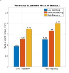
Fig. 16. Result of Resistance of trajectory tracking experiment of subject 2. Similarly, the fast trajectory and high damping condition contribute to the highest resistance torque of 2.00 Nm.
