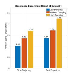
Fig. 15. Result of Resistance of trajectory tracking experiment of subject 1. The height of bar graph denotes the RMS value of measured joint torque. The highest resistance torque occurs at the fast trajectory and high damping condition with the value of 2.25 Nm.
