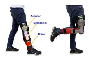
Fig. 1. The proposed knee exoskeleton with mechanical components and its range of motion during the walking stage.
