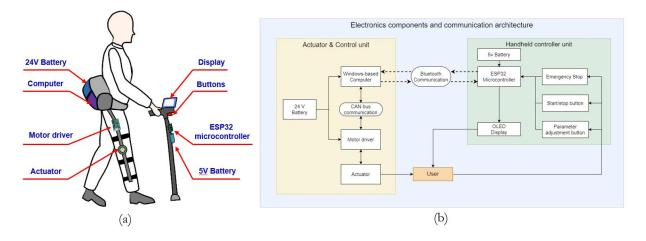
Fig. 6. Electronic components and communication architecture of the proposed robot system. (a) Electronic components of two subunits: Actuator & Control unit and Handheld controller unit. (b) Communication flow and use diagram of the robot system.
