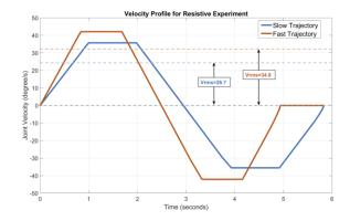
Fig. 14. The fast trajectory (red) and the slow trajectory (blue). The slow trajectory has an RMS velocity of 26.7 deg/s, while the fast trajectory has an RMS velocity of 34.8 deg/s.
