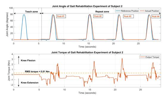
Fig. 19. The result of the Gait Rehabilitation Experiment of subject 2. The RMS torque is 0.81 Nm occurred during the peak angle of the knee flexion.
