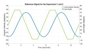
Fig. 10. Trapezoidal velocity profile and corresponding position signal. The maximum joint angular velocity and position is 39.0 degree/s and 70 degrees respectively. Each cycle takes 5.80 seconds to complete.
