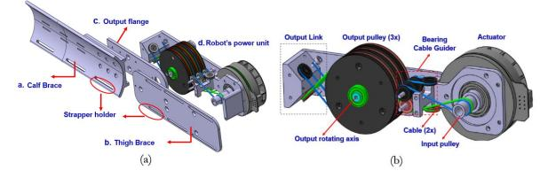
Fig. 2. Mechanical design and components used in the proposed robot. (a) overall components. (b) the novel cabledriven transmission mechanism.
