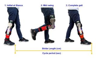
Fig. 17. Experimental setup and parameters employed in the computation for gait rehabilitation. The stride length and cycle period are determined using the length and time frame from the initial to the completion of gait.
