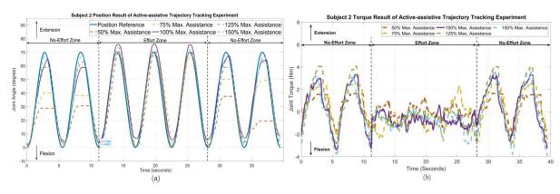
Fig. 13. Results of the active-assistive trajectory tracking experiment of subject 2. The based-torque (100% Max. Assistance) for subject 2 is 3.0 Nm. (a) the joint angle of subject 2 in the experiment. (b) the joint torque of subject 2 corresponding to the position reference.
