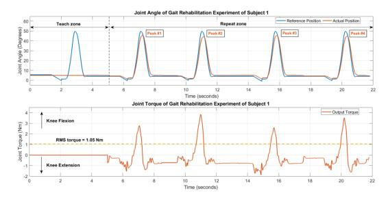
Fig. 18. The result of the Gait Rehabilitation Experiment of subject 1. The RMS torque is 1.05 Nm and occurred during the peak angle of the knee flexion.
