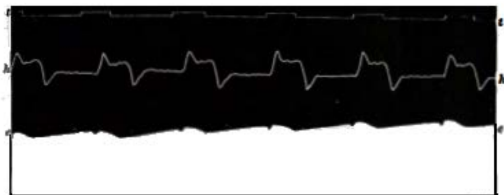
FIG. 1. Man. Heart led off to electrometer from front and back of chest (front to Hg; back to H_2SO_4 ). e.e. electrometer. h.h. cardiograph. t.t. time in seconds.
