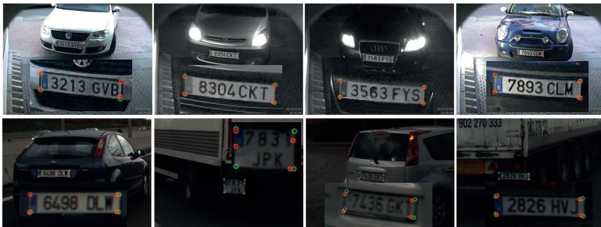
Figure A.4: Examples of license plate corners detection on the validation set (top row) and on the test set (bottom row). Green circles are the ground truth, red circles are the predictions. License plate area has been zoomed to ease visualisation.
