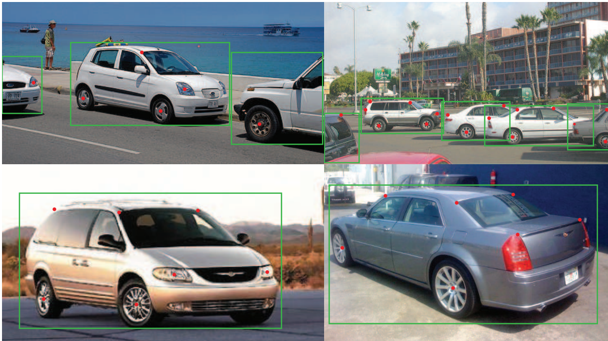
Figure 3.4: Example of some of the images from PASCAL3D+. In green the bounding boxes and in red the keypoints. Top row images are from PASCAL and bottom ones from ImageNet.
