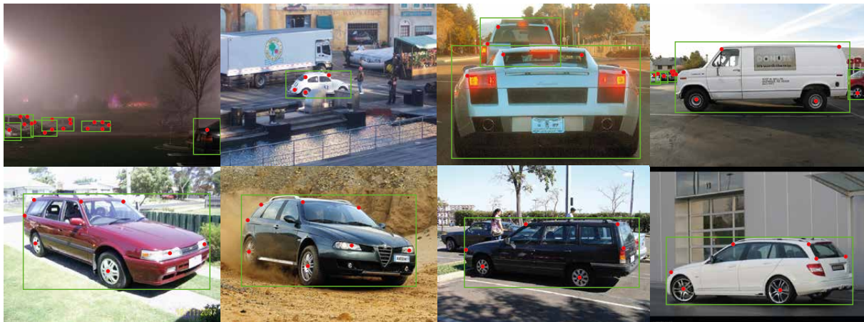
Figure 2.1: Example of some of the images from PASCAL3D+ dataset. In green the bounding boxes and in red the keypoints. Top row images are from PASCAL subset and bottom ones from ImageNet subset.
