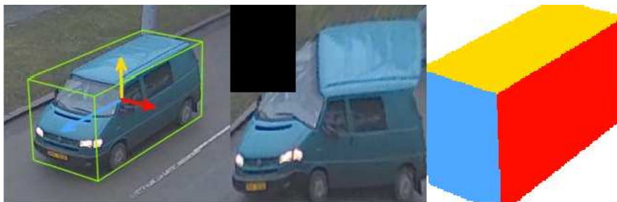
Figure 2.14: Visual example of the 3D bounding box used by Sochor et al. [5] to unpack vehicle shapes and orientation.
