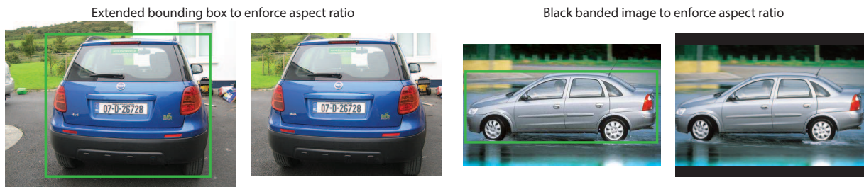
Figure 3.1: Aspect ratio enforcement examples. Extended bounding box on the left and black banded on the right.
