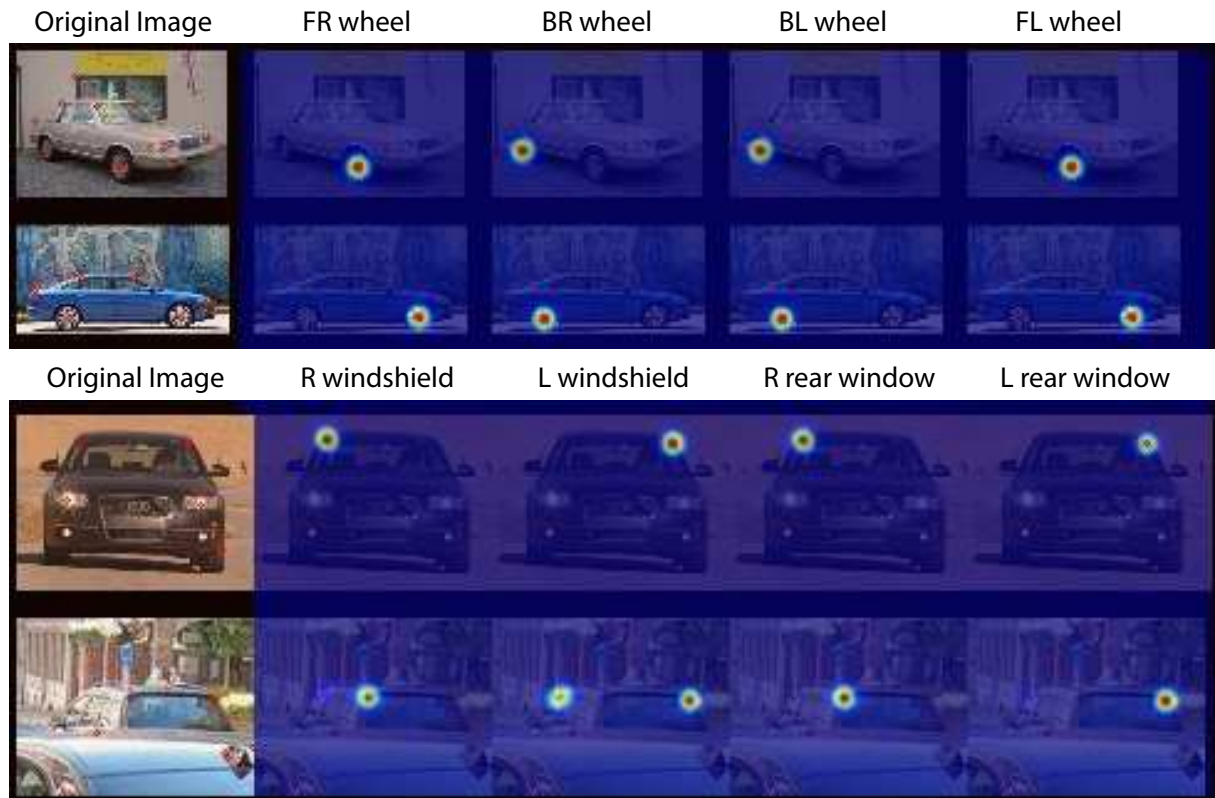
Figure 5.6: Output heatmaps for SBVPE-PASCAL3D+/PASCAL. Examples of the keypoint confusion phenomenon for the wheels (first and second row) and the windshield/rear window (third and fourth rows). For the first and second rows the second and third columns show the correct wheels prediction while the fourth and fifth columns show incorrectly predicted ones. For the third row the second and third columns show correctly predicted windshield corners while the fourth and fifth columns show incorrectly predicted rear window corners. For the fourth row second and third columns show incorrectly predicted windshield corners while the fourth and fifth columns show correctly predicted rear windows ones.
