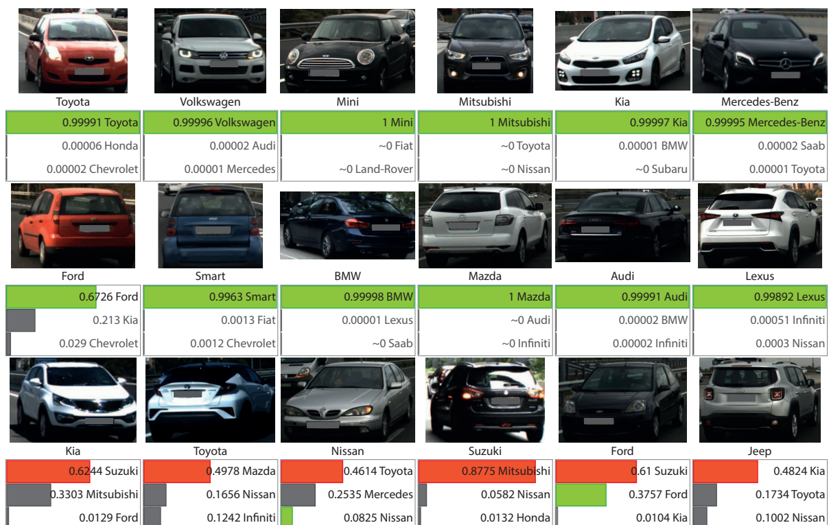
Figure 5.19: Top3 predicted classes of the Fusion-Makers trained model for sample images from the PREVENTION Makers test set. The first row shows correctly classified front view images. The middle row shows correctly classified rear view images. The bottom row shows misclassified images from both views.
