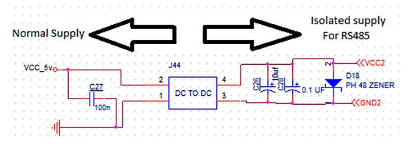
Figure 6. MMCA – RS485 DC to DC isolated power supply.
