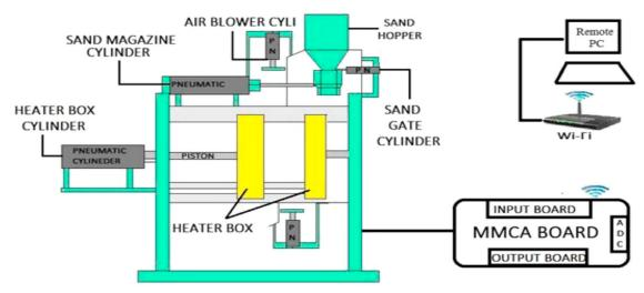
Figure 1. Block diagram of the CSM.
