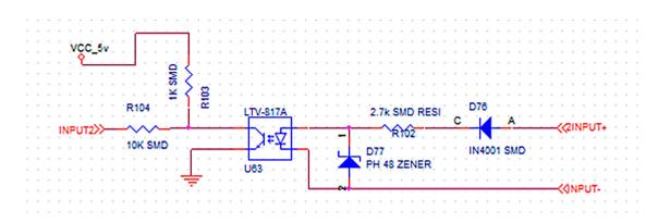
Figure 9. MMCA 24 V input circuit.
