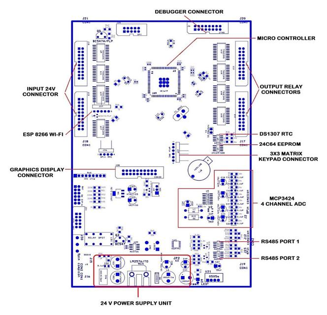
Figure 4. MMCA PCB (front view).
