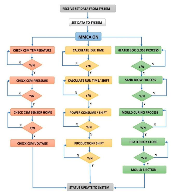
Figure 3. Programming logic for CSM.
