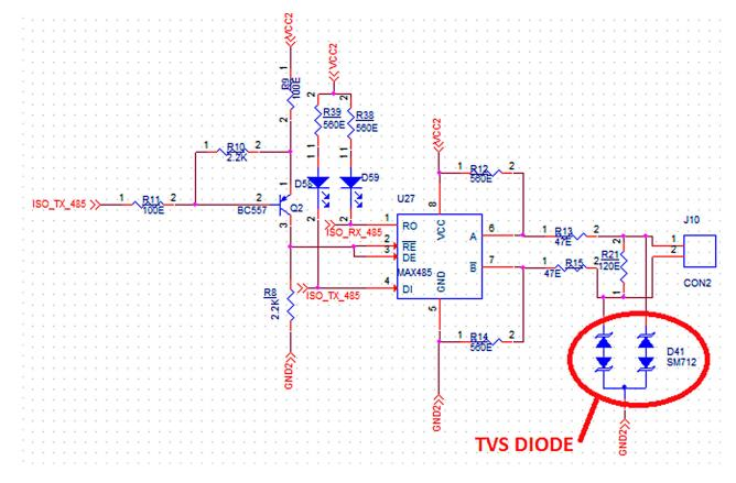
Figure 7. Isolated RS485 circuit and TVS diode.
