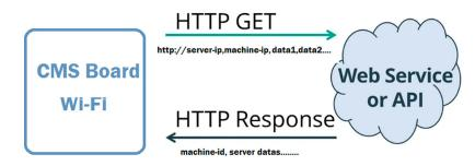
Figure 11. Block diagram of HTTP request and response.
