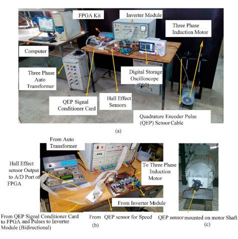
Figure 9. (a) Experimental setup for the proposed DTC-IM drive. (b) Peripheral connections of FPGA. (c) QEP sensor mounted on motor shaft.
