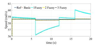
**Figure 16.** Speed responses of basic, 1fuzzy, 2fuzzy and 3fuzzy DTC schemes for a speed reference of 58.612 rad/s.
