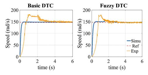
Figure 11. Speed responses of basic and fuzzy DTC schemes during starting.
