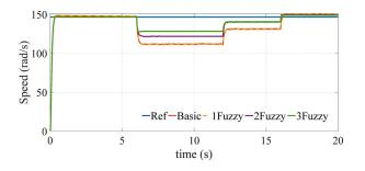
**Figure 15.** Speed responses of basic, 1fuzzy, 2fuzzy and 3fuzzy DTC schemes for a speed reference of 146.53 rad/s.
