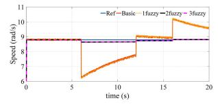
**Figure 17.** Speed responses of basic, 1fuzzy, 2fuzzy and 3fuzzy DTC schemes for a speed reference of 8.7912 rad/s.
