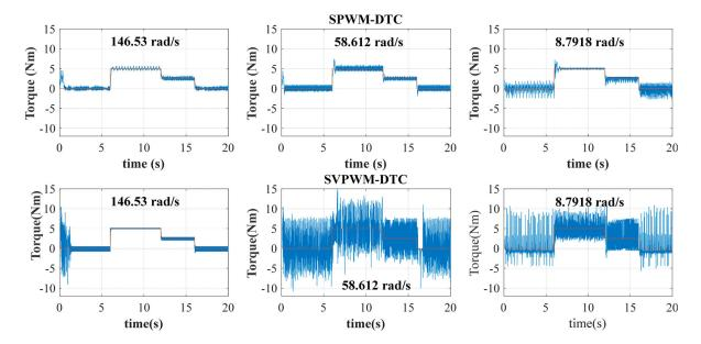
Figure 14. Torque responses of SPWM-DTC and SVPWM-DTC schemes for a speed reference of 146.53, 51.612 and 8.7912 rad/s.
