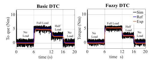
Figure 10. Torque responses of basic and fuzzy DTC schemes.
