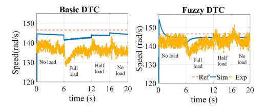
Figure 12. Steady-state speed responses of basic and fuzzy DTC schemes: full load, half load and no load.
