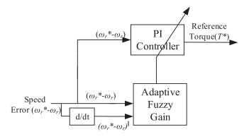
Figure 6. Block diagram of FGS tuned PI speed controller.
