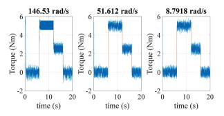
**Figure 18.** Torque responses of fuzzy DTC (3fuzzy) schemes for a speed reference of 146.53, 51.612 and 8.7912 rad/s.
