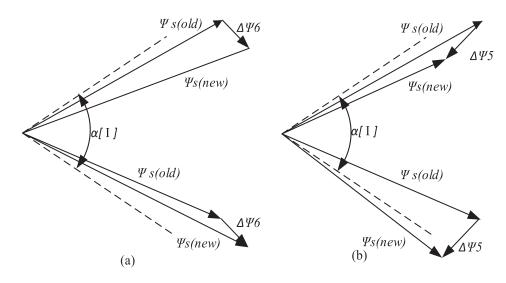
Figure 3. Uneven voltage vector contribution in sector I. (a) For voltage vector U6 and (b) for voltage vector U5.
