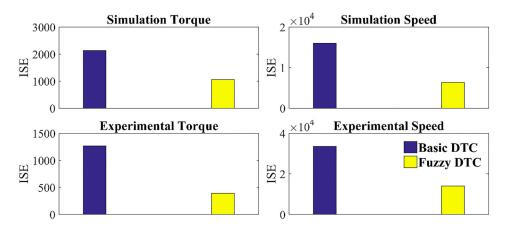
Figure 19. Bar chart representation of the performance index ISE for speed and torque error from simulation and experimental studies.
