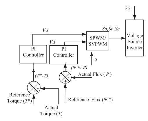
Figure 4. SPWM/SVPWM for DTC.
