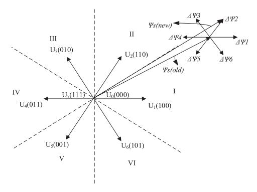
Figure 2. Stator flux plot and voltage vectors in conventional DTC.
