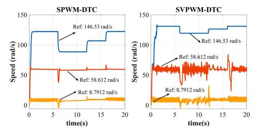
Figure 13. Speed responses of SPWM-DTC and SVPWM-DTC schemes for a speed reference of 146.53, 51.612 and 8.7912 rad/s.
