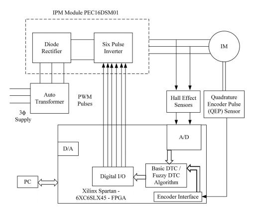
Figure 8. Schematic diagram of experimental setup for the DTC-IM drive.
