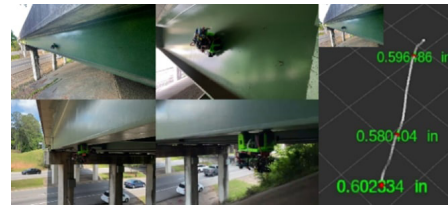
Fig. 6. Real-time synchronization of robot positioning and thickness measurement on a bridge near LaGrange, GA, USA - robot path in white color, thickness measurement points in red dots, and thickness readings in green color.
