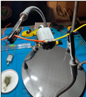
Fig 6. TT DC motors soldered to electrical wires
