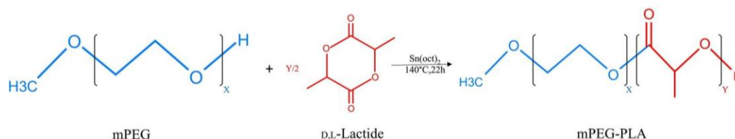
Figure 9: AB diblock formation via ring-opening polymerization of D,L-lactide and methoxypolyethylene glycol 32
