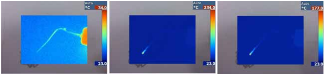
Fig. (3). Temperature profiles along the heat pluggers detected from the thermal imaging camera. (A) Profile of the heat plugger before heating; (B) profile of the heat plugger after heating with System B; and (C) profile of the heat plugger after heating with System MB.
